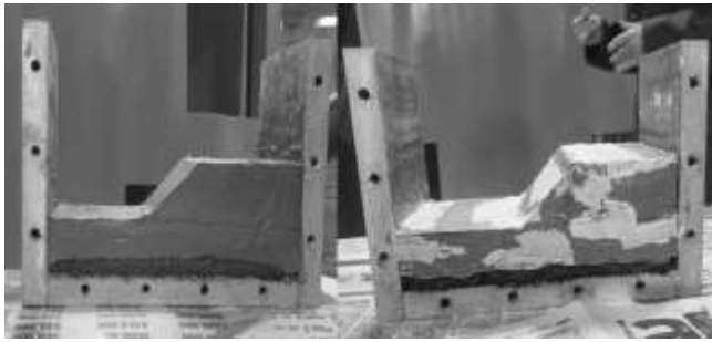
Figure 4. Laboratory models of the MAGE graduate course: a) Homogeneous soil slope; b) Heterogeneous soil slope. Source: The authors.
